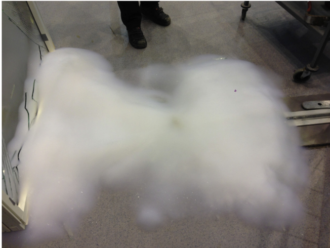
Fig. 10. Photograph of an accidentally broken AGU. Aerogel granules have been scattered in a large area.
