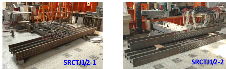
(a) Different arrangements of the shear studs
