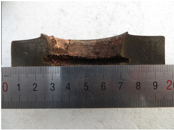
Fig. 3. Profile of steel plate after penetrated by radial jet cracker.
